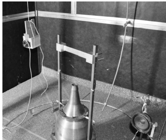
VKI Jet-airfoil interaction noise facility
